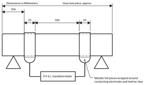
Figure 6-1 - Electrodes and contacts for testing hose
