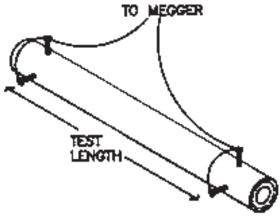
Figure 6-2 - Nail or "Pot Room" Test
