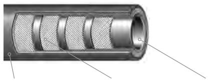
Cover The cover is the outermost or visible area of the hose. It is designed to be a protective covering against wear, abrasion, cuts, weather, and the general destructive action encountered in normal service. Body or Carcass The body reinforcement is the supporting structure of the hose. It can range from simple to complex combinations and consists of cord, yarn, fabric, wire or any combination of these.
